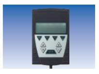
The HMI of SICLIMAT®-SAPHIR can be used as a handheld terminal, but can also be mounted in a control panel. If has a display with 4 lines each with 20 characters, which offers convenient and easy-to-understand operation with the menu and function buttons. An integrated red alarm LED instantly indicates operational faults.
